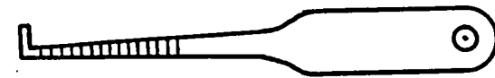
Figure 9C. With a carbide-tip tool engraver, meter your lock pick "J" for picking rotary tumbler locks. Etch lines .050" apart.
